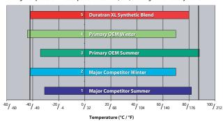
\*Minimum viscosity is 9.1cSt @ 100°C. The after-shear temperature at 9.1cSt shows the stability of the fluid (higher is better).
