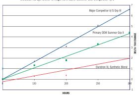
\*Note: Results are after 300 hr ABOT Oxidation Test which is more severe than JD requirement Allison C-4 ( GM 6137M) Oxidation Test.
