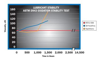
REFLO A's strong oxidation stability guards against fluid breakdown in systems where air or oxygen contamination is an issue. Fewer fluid change-outs can reduce costly downtime.
