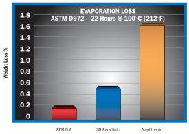
REFLO A's lower oil volatility significantly reduces the oil carryover experienced with solvent refined paraffinic and naphthenic fluids.
